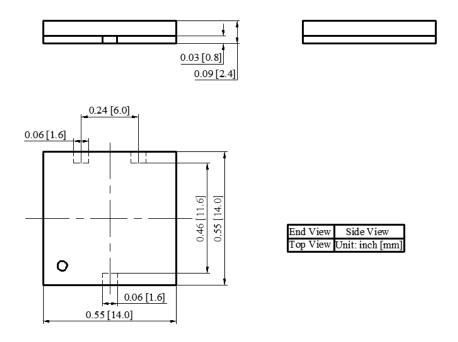
Figure 3. Dimensions of the Voltage Reference
