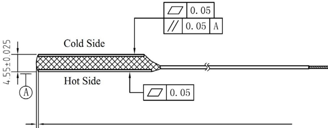
The head of the RTV sealing shall be 0.5 maximum out of the module's edge, except for where near the soldered ends of the lead wire.
