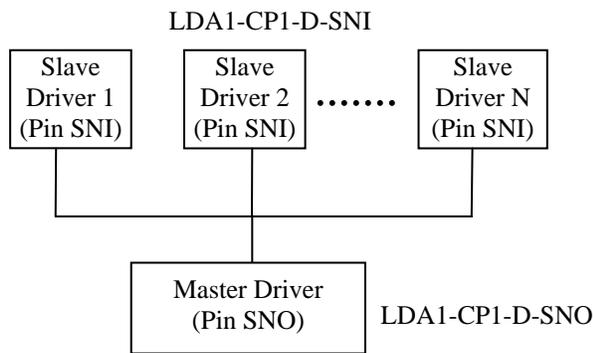
Figure 4. Schematic for Applications Using Multiple Drivers
