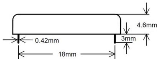
Figure 9. End View of LDA1-CP1-D
